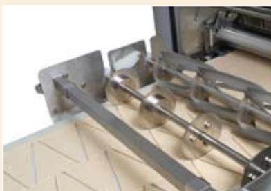
This regulator allows for the appropriate control of the belt speed for dough cutting or a dough transfer of 2-7 m/min.
