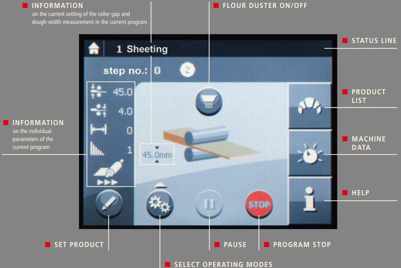
The modern computer control of a FRITSCH ROLLFIX (like that of the ROLLFIX 600 or the ROLLFIX 700) will add greater convenience and routine to your daily work. You put the dough on the infeed table and select the appropriate program – then the ROLLFIX does all the rest. A user-friendly tilted display keeps you informed at all times about the state of things – and in plain words („puff pastry dough“, for example) and with self-explanatory graphics.
