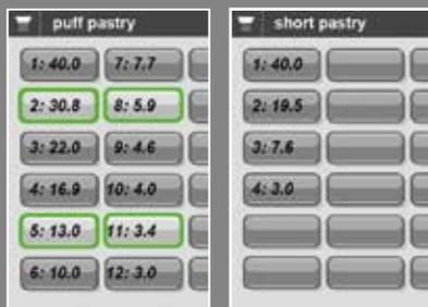
In this detailed view of the individual dough sheeting reduction curves, you see not only the number and sequence of the dough sheeting steps but also with the help of the green highlighting at which stage of sheeting the flour duster is switched on.
