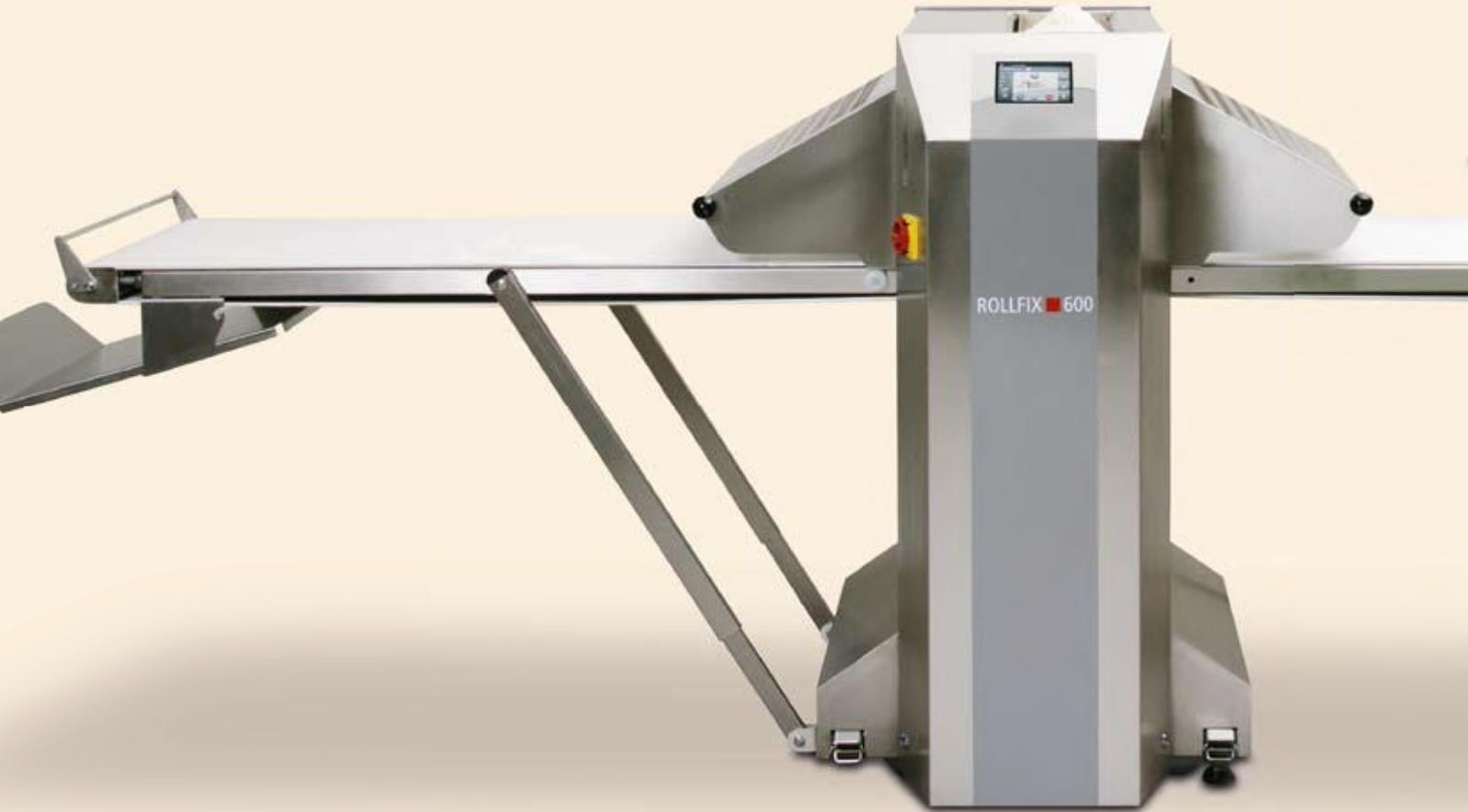
ROLLFIX 600 with flour duster, fully-automatic dough-spooling unit and long table.
