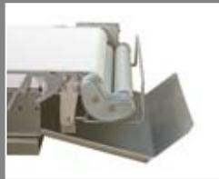
Out of the way when not in use, yet automatically called up for duty when needed: the fully-automatic dough spooling unit.
