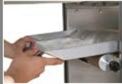
The waste flour container prevents the accumulation of dirt inside the unit and can easily be removed for cleaning.
