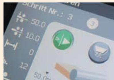
Super practical: The „slow motion“ switch allows you to quickly reduce the speed of the infeed conveyor. Thus the dough is quickly transported onwards from the exit table preventing possible accumulation of dough or rippled dough sheets.
