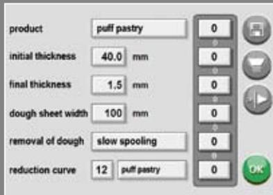
Here's how easy it is to set up a dough sheeting program for a specific dough type: via a standard computer keyboard you call up the name of the product onto the monitor and then enter the beginning and final thickness values and the desired dough width.
